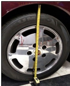
14+ inch wheel measurement of a stock 16-inch wheel and stock suspension set up.
