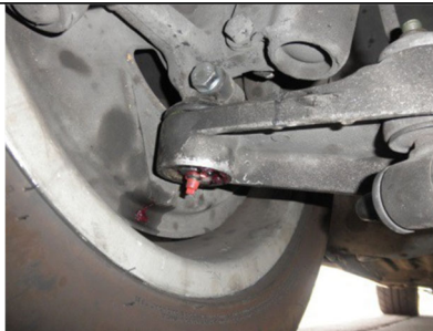
Late 944 aluminum arm with rebuilt ball joint.
