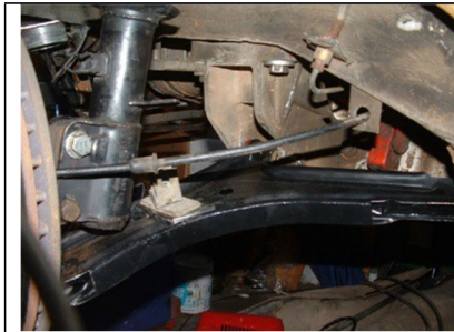
Early 944 steel arm with reinforcements.
