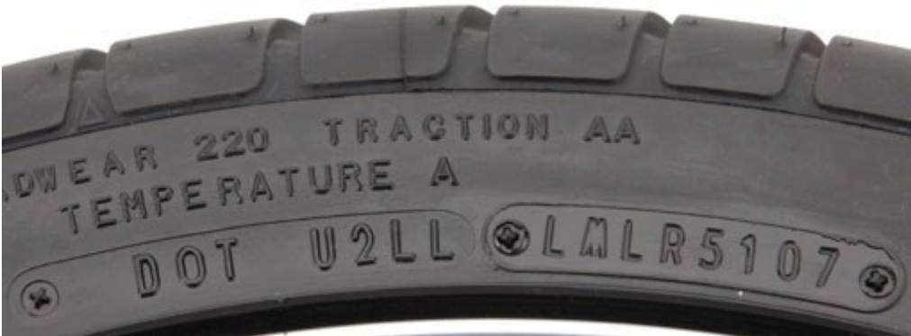
(Tire date of manufacture as stamped into the side wall)
