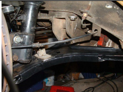
Early 944 steel arm with reinforcements.
