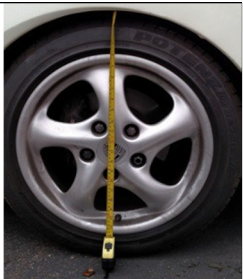
13.2 inch wheel measurement of a car with lowering springs and 17 inch wheels.
