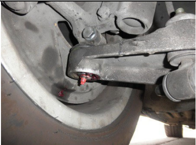
Late 944 aluminum arm with rebuilt ball joint.
