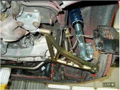
Tubular racing arms (Fabcar or equivalent).
